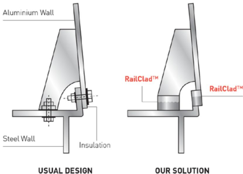
Explosion welding can replace conventional bolted joints.
