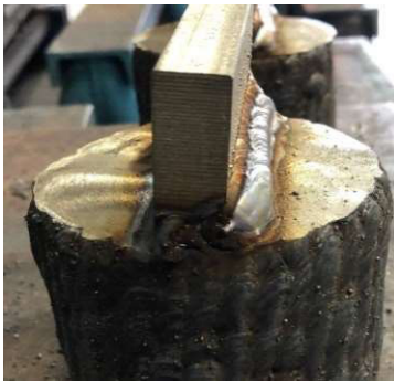
Figure 5: ASTM G146 Specimen for DirectAttach™
