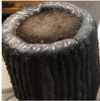
Figure 4: ASTM G146 Specimen Weld Overlaid on the Edge
