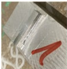
Figure 6: Specimen 1 sheared off in the interface
