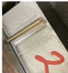
Figure 7: Specimen 2 sheared off in the 470LI
